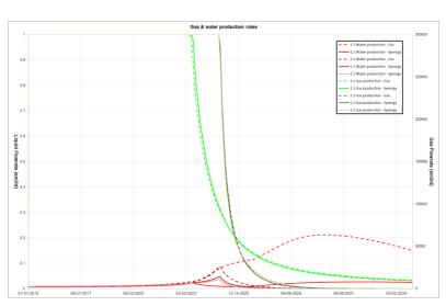
Fig. 2: Gas and water production rates of the gas well. Case 1: Boskoop properties, case 2: high permeability, case 3: high permeability and higher doublet rate.
