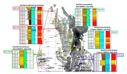
*Fig. 5:* Regional reservoir architecture – typical well log response for different types of Volpriehausen sandstone (*RBMVL*). Study area is outlined in solid black, yellow polygons indicate Triassic leads. In both the A05-01 and Bertel-01 there is an age-dating uncertainty for the Triassic rocks. Analyses of biostratigraphy, heavy minerals, clay mineralogy, grain size distributions and guartz surface microtextures on cuttings and core material from the Dutch northern offshore
