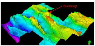
*Fig. 1: Structure of the Boskoop field and surrounding area. Surface from seismic interpretation, base Altena.*
