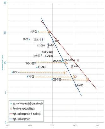
Fig. 3: Porosity depth trends. Porosity vs present depth, porosity vs max burial depth and suggestions for max porosity envelopes.
