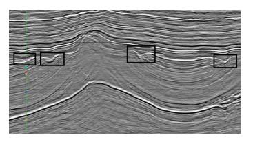
Fig. 1 Subrosional sinks of Triassic evaporites below the Late Cimmerian unconformity (c. Base Lower Cretaceous) near the German border in the NL part of the North Sea.
