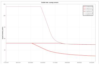
Fig. 3: During a synergy scenario the doublet rates cannot be maintained due to the declining reservoir pressure.
